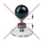
2. You can push the gauge down to the round metal stop with the metal shim in place.
