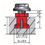
D<sub>1</sub> = hole diameter (dia. 7 mm)
