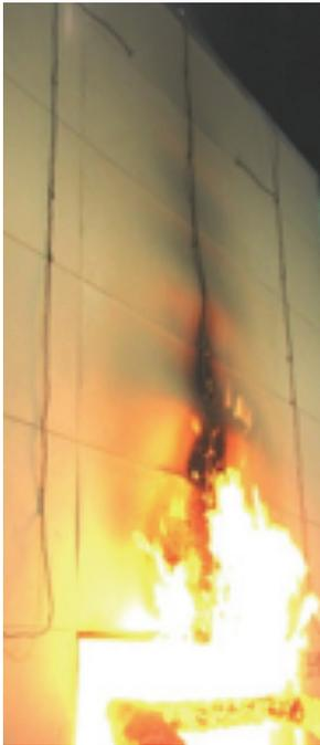
Figure 19 – NFPA 285 -Post Test
